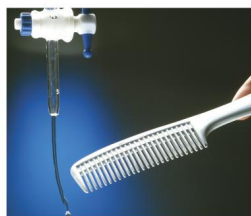
▲ You can bend a stream of water with static electricity.
