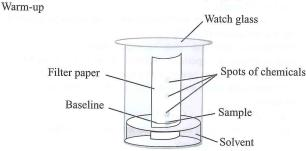
1.1 E:  $R_f = \frac{\text{distance travelled by substance}}{\text{distance travelled by solvent}} = \frac{3.6}{9.5} = 0.38$
