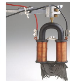
▲ The strength of an electromagnet depends on the number of turns on the coil, the current, and the core.
