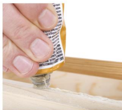
▲ Evaporation makes some glues dry. The solvent evaporates. A sticky substance remains, joining the surfaces.
