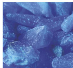
▲ Copper sulfate crystals. The more slowly the water evaporates, the bigger the crystals formed.
